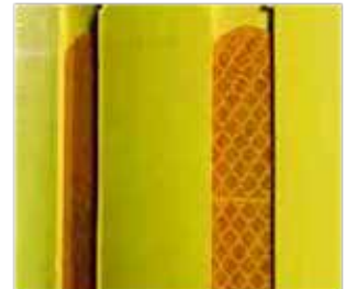
Light reflectors External reflectors in the upper part of the buoy.
